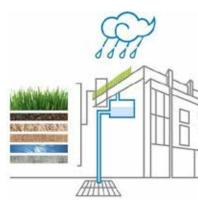
In addition to the landscaped terrace at the building entrance, Hunter Terrace will feature select areas of green roof to retain water and add insulation to the roof. Due to concerns over long term durability and maintenance, the development team will be selective in the areas to which green roofs are applied.
