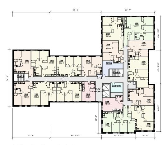
3rd Floor Plan Diagram (typical)
